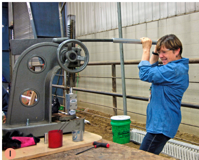
Wanda Garrett compressing fuel into a rocket with a large press.
