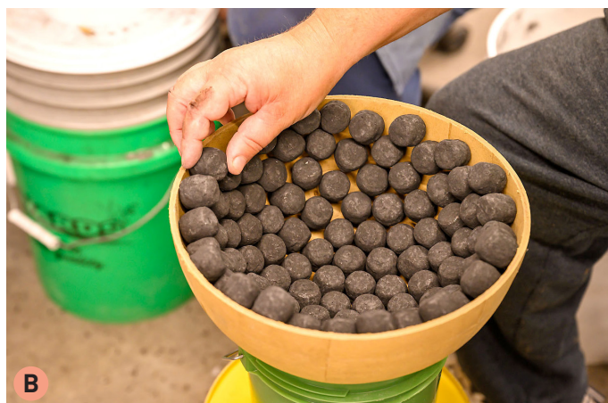
Placing stars in a hemi for a large shell.
