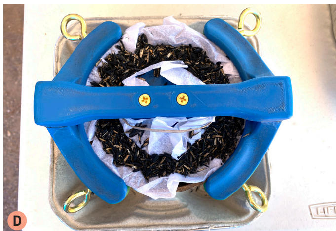
A 3D-printed jig allows compaction of burst powder over the outer petal of stars, saving space for the inner petal.
