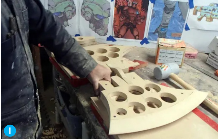
The blades propped up on some scraps of MDF so they'll stay straight
