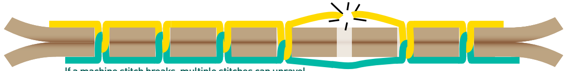
If a machine stitch breaks, multiple stitches can unravel
