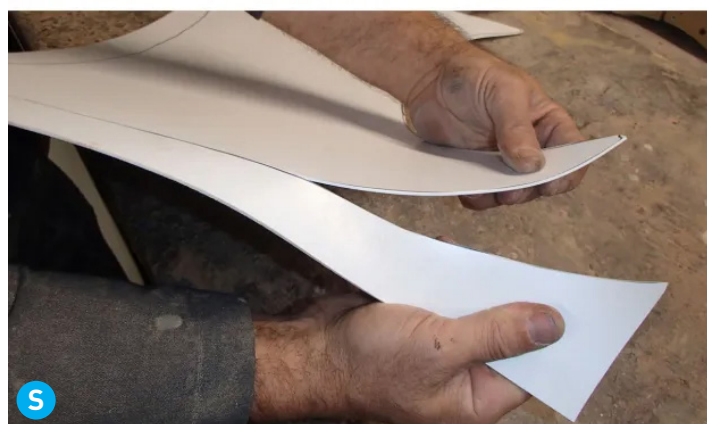
Score and snap — the quick and easy way to get shapes out of styrene
