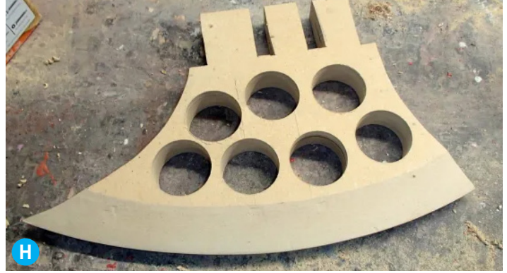
The hole saw quickly makes Swiss cheese out of the MDF axe blade.
