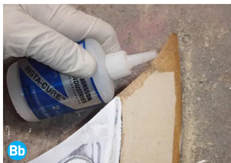
Soaking the edges of the blade with cyanoacrylate glue for strength
