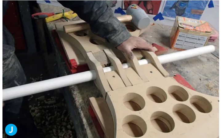
Keeping the handle in place makes sure that the holes will line up properly.
