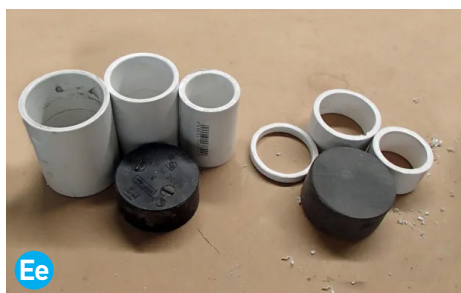
Boring pipe fittings (left) stop being recognizable (right) with just a bit of love from a miter saw and a sanding block.
