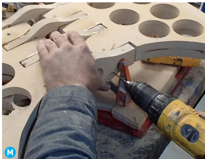
The pre-drilled hole will make it possible for the screw to effortlessly penetrate the MDF without splitting it apart.
