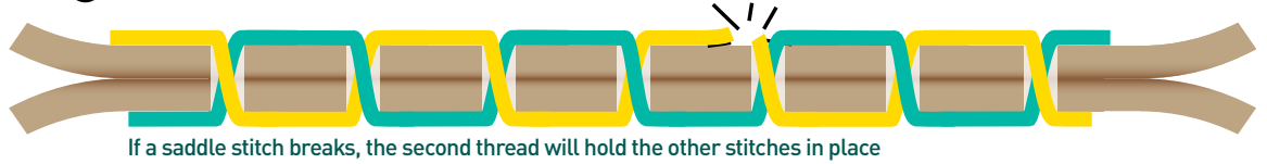
If a saddle stitch breaks, the second thread will hold the other stitches in place
