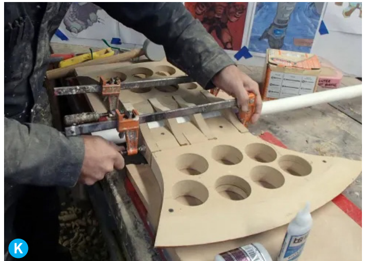
These are bar clamps, just one of the countless varieties of clamps that you will need more of.
