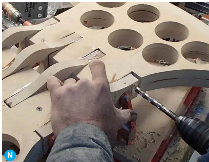
Making a bigger hole for the screw head to hide in is called "countersinking."
