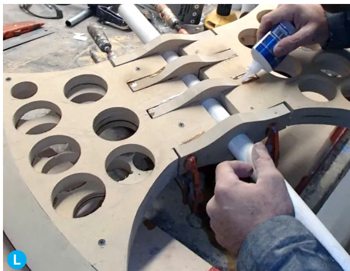
Applying glue to the seams
